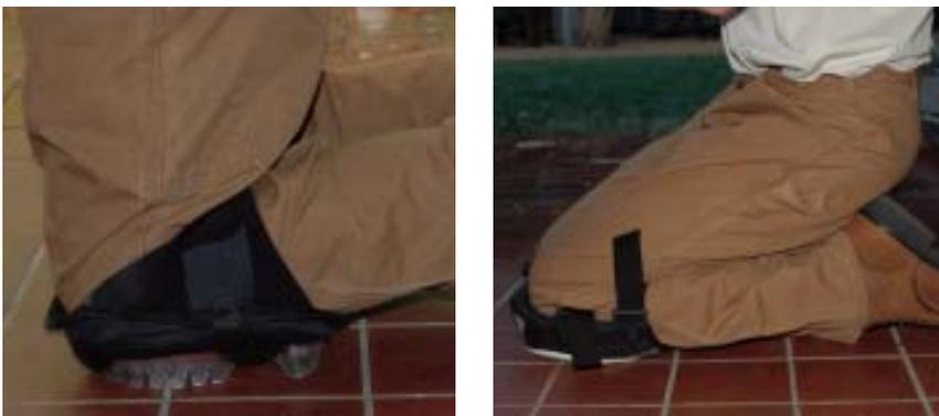
**Figure 2.** Flat and concave soft-cap models (left) provide excellent stability because they bear flat against the ground. With curved caps (right), it's easy to roll forward and from side to side; if the caps are thin, it's more comfortable to lean back and kneel-sit.
